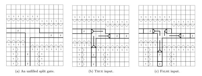
Figure 8: A split gate unfilled and filled with both truth values.
