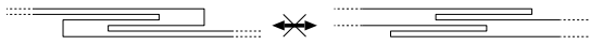
Figure 4: Two legal folded states for a string which cannot be exchanged by local simple (un)foldings.
