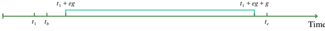
Figure 4: The entity leaves a square at t_b and returns at t_e . If t_e - t_b is larger than g + g\epsilon , there is a snapshot in which the entity is outside the square.
