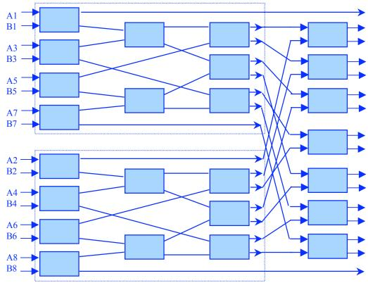
Now we combine the necessary stages of the merge network to implement the sort in the same way as was done in class for the 4 element networks.
