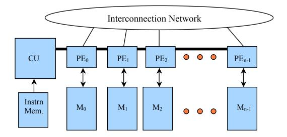
In general, APs are likely to be more scalable and therefore offer more potential parallelism. Of course, this will depend on the problem being solved being able to make use of the parallelism offered. The parallelism provided in one D-Unit pipeline in a PVP is limited by the number of stages in the pipeline. Further, there is unlikely to be sufficient ILP to keep very many D-Unit pipelines busy.
