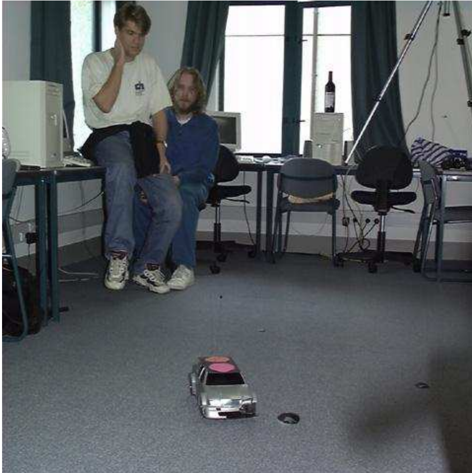
Fig. 1. Aucklandianapolis at the University of Auckland. The tripod of the vision system can be seen on the top right corner of the image. The video camera is just out of the picture. The video server determines position and orientation of the cars by bright dots on the car. As can be seen, the speed trials took their toll on our cars.
