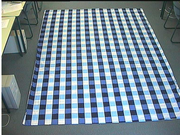
Fig. 2. Calibration Pattern as seen by the Camera
