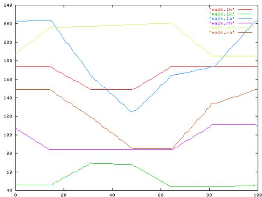
Figure 4: Servo Settings for a Straight Walk
