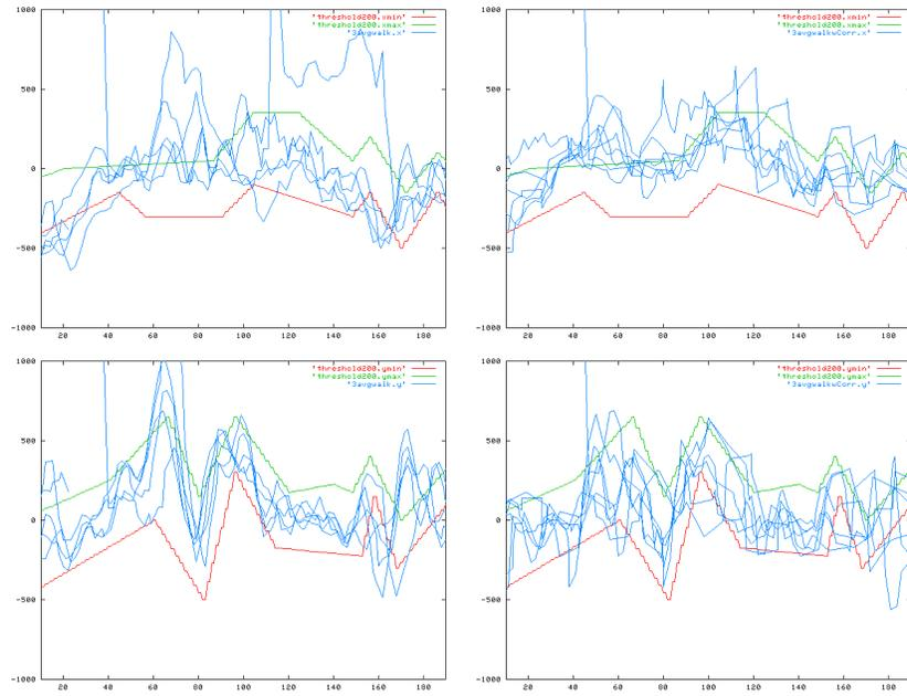
**Fig. 4.** Comparison of original walking gait (left column) and walking gait with motion compensation (right column) in the saggital (top row) and lateral (bottom row) plane.
