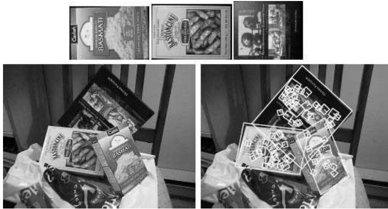
Fig. 2. Using SIFT the sample objects(above) are searched from in the image(left). The keys generated are used to match the samples to the image(right). Images are from [6].
