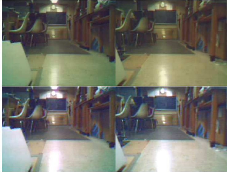
Fig. 7. The normalization process helps balance the colours in the image by stretching the colour range of pixels.
