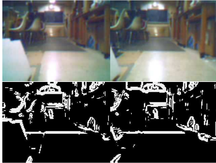
Fig. 9. The result of applying a Sobel edge detection to the blurred image.
