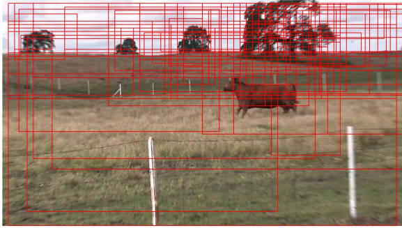
Figure 2. An example of generating object proposals. Given an frame in a video, the objectness in [23] is applied. It returns a collection of bounding boxes in the image that are likely to be any objects. For each bounding box, the objectness also assigns a score indicating how likely it is to be an object.
